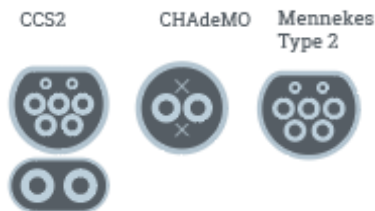
Configuration of charging ports on CCS, CHAdeMO and Type 2 connectors (Designability)
